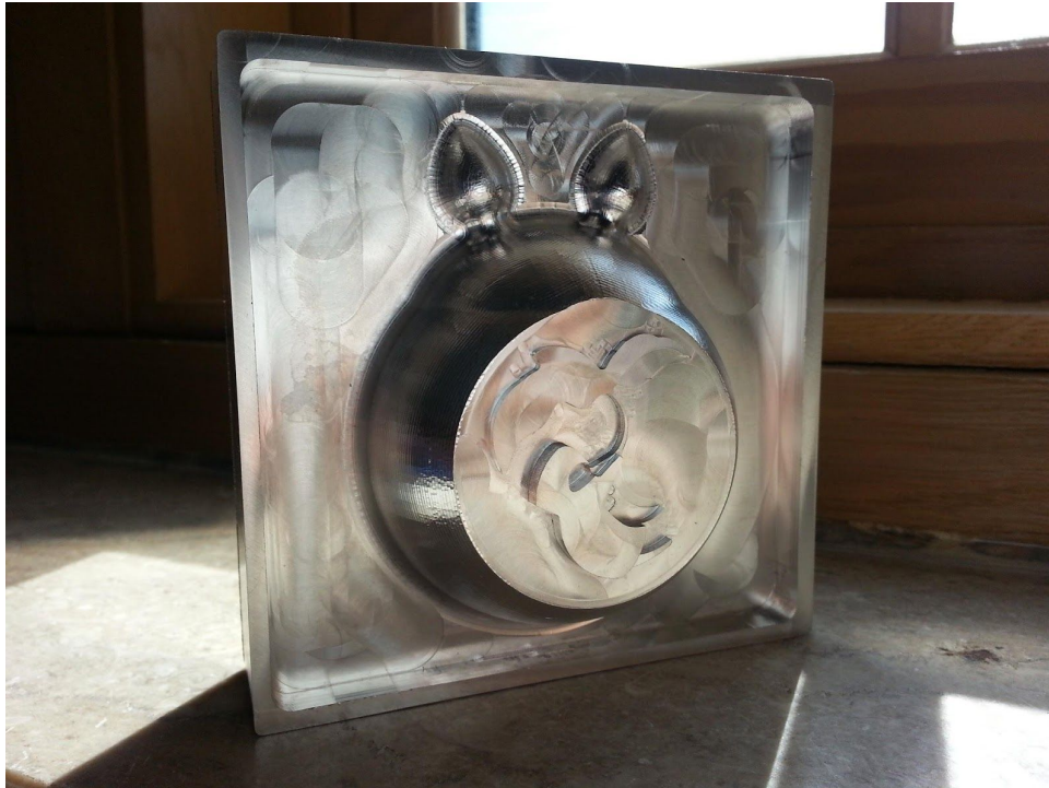
Figure 20: The cleaned but unpolished final aluminum part
